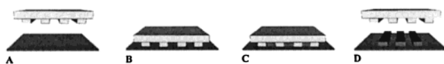
Figure 5. Schematic of the procedure used in MIMIC. A PDMS stamp is placed onto a substrate (A and B). A drop of the polymer solution is placed in contact with the stamp and substrate, and the channels are filled by capillary action (C). After evaporation of the solvent, the stamp is removed and the polymer remains on the substrate (D).
